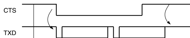
Figure 34-29. Transmitter Behavior when Operating with Hardware Handshaking
